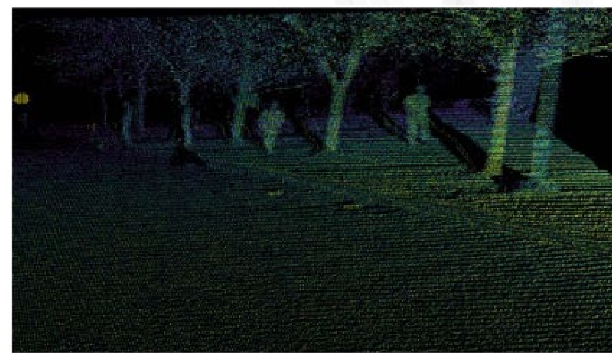
Insight LiDAR – Ultra High Res (0.025 x 0.025 deg) Bricks in the road and pedestrians clearly visible
